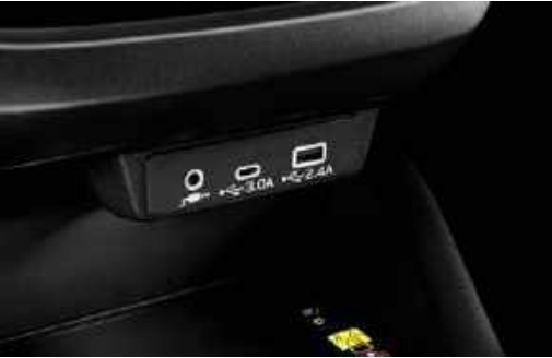
Front USB Ports (Type-A and C*2) and Rear USB Power Ports*2
